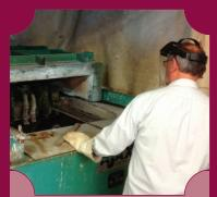
Our dip-brazing pot and induction brazing are used for both aluminum and copper alloys as well as silver brazing for thin wall space qualified assemblies.
