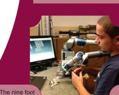
laser FARO "Edge" 7 axis measurement arm is the most advanced FaroArm available. This arm allows easy verification of product by inspecting tooling, CAD analysis and reverse engineering. FARO "Edge" takes portable metrology to the next level.
