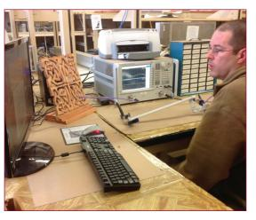
A vector network analyzer, the Agilent N5235A PNA, measures parameters, including VSWR, insertion loss, coupling and directivity from 10MHz to 50GHz. A -110 dB noise floor and 33,000 data point capacity, offers signal sensitivity and data resolution, allowing the convenience and flexibility of digital data in a variety of formats.
