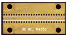
Board Ø (2003) Serial Number = Ø Trace = 0.045" Ground = 0.064" Via Size = 0.020" Via Spacing = 0.040" Via Rows = 0.112" Fabricated = 2003
