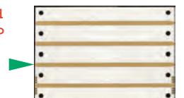
Straight microstrip test board 20c, S/N 54
