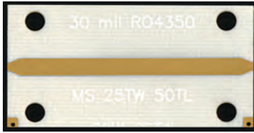
Straight microstrip test board 15c, 30 mil R04350, S/N = 51, (with actual test results).
