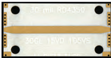
Top ground launch microstrip test board 14c, 30 mil R04350, S/N = 52, (with actual test results).
