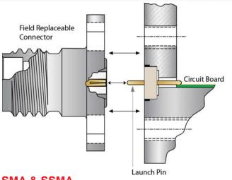
Field Serviceable Connectors for better reliability and performance. SMI accessories are separate from the connector and provide the following benefits:
