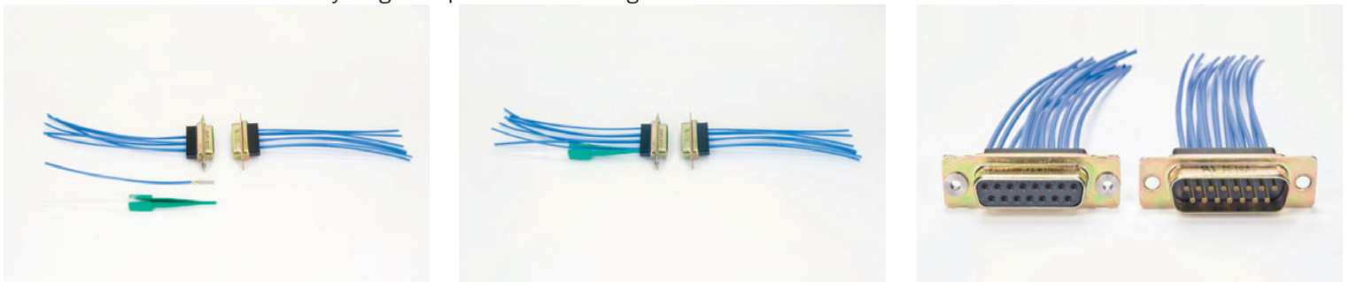
Figure 5: Installation sequence for inserting SSBP coaxes into a D-Sub connector.
