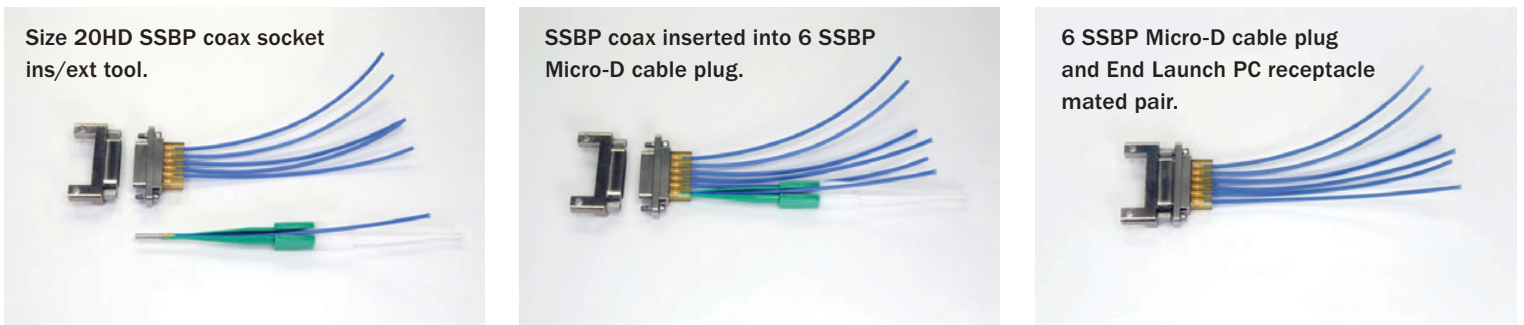
Figure 9: Installation sequence for inserting SSBP coaxes into a Micro-D connector.
