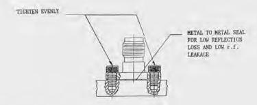
For example, a possible sequence for screw-tightening a 4-hole mount connector could be the following:
